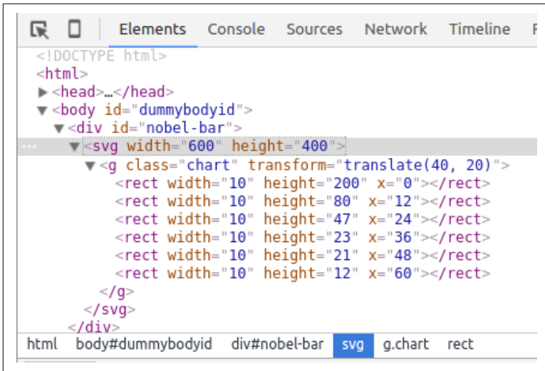
Figure 16-14. Using the Elements tab to see the HTML generated by enter and append
